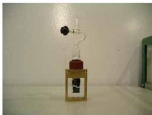
Fig. 1. Photograph of the sample vessel which is mounted on cell fixer. The sample powder of 5 – 10 μm is inserted in the gap of 100 μm of the vessel in support of ultrasonic apparatus.
