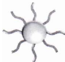
Fig.1. Schematic drawing of surface-modified silica nano-particle with polymer brushes.
