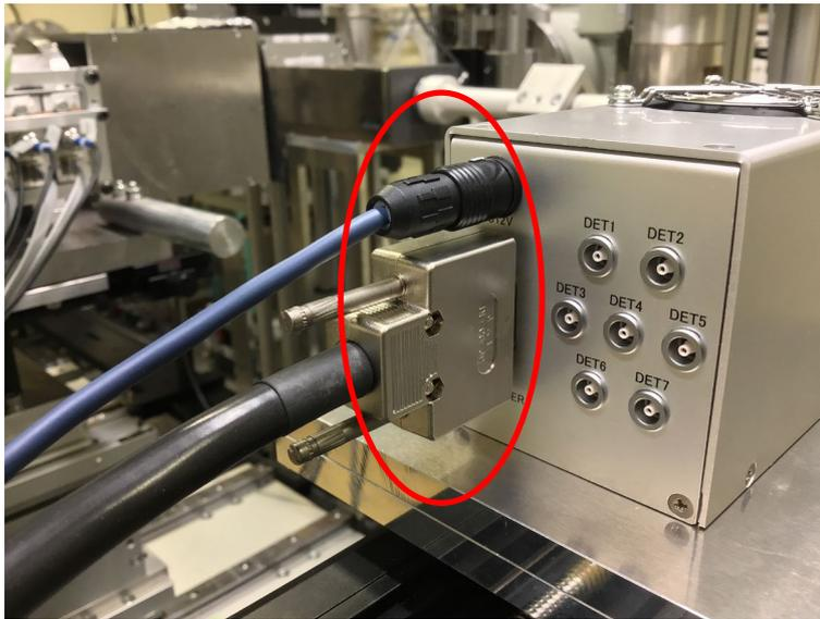
(4) Connect the signal cables to the 7-element SDD. Each connector number (DEC1-7) is labeled on each signal cable.
